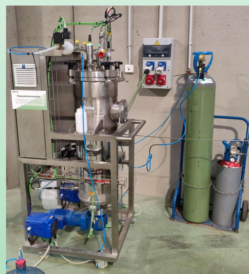
Figure 3: Hybrid fermentation system for biopolymers and biochemicals production from biogenic CO 2 .
